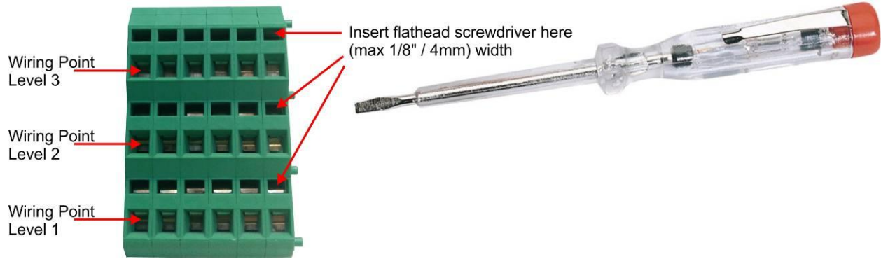
Figure 1.2: Terminal Wiring Details
