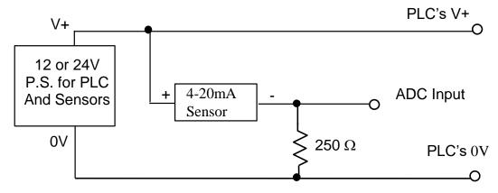
For ADC #7 & #8, use a 253.16 ohm resistor instead of 250 ohms as explained in 5.2.2.
