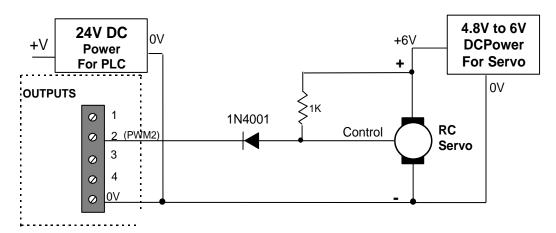
Figure 11.4 Non-isolated Interace to RC Servo
