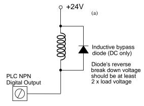
Figure 1.7 – Protective Solid State Output Against Inductive Kick.
