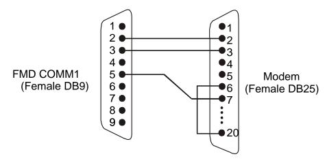
Figure 14.3 Connecting FMD1616-10's COMM1 to a modem's DB25 port
