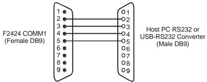
Figure 14.1 Connecting COMM1 with PC
