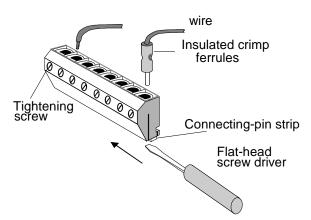
Figure 1.3 - Removing Screw Terminal block
