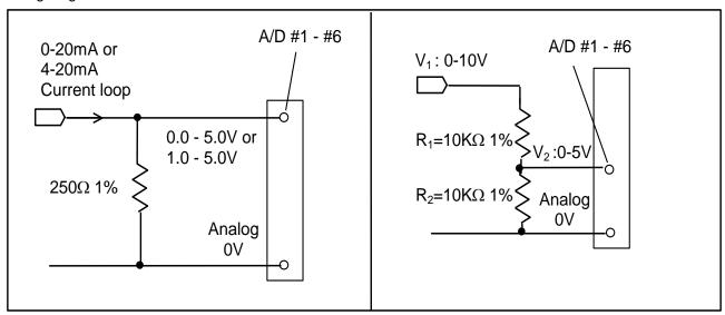
Converting 20mA current-loop to 0-5V
