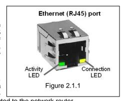
Once connected to the network, the TRiLOGI programming software and TRi-ExcelLink works instantaneously with the PLC, allowing remote programming and process monitoring over the LAN or the Internet. In addition, the Ethernet facility at this port can host web pages and Java applets so that users of the equipment can control/monitor their equipment using their web browser from anywhere.
