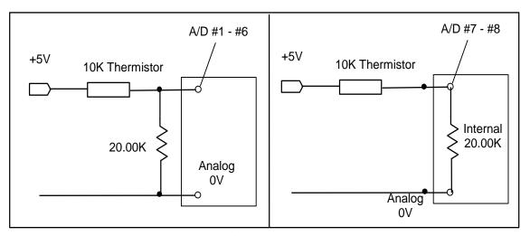
Connecting 10K Thermistor to ADC 1-6
