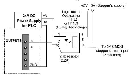
Figure 10.2 Conversion of FMD1616-10 outputs to 5V logic level
