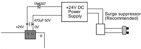
To ensure that the power supply provides a slow voltage gradient during power down, the power switch must be connected to the AC side of the power supply instead of to the DC side of the power supply. All industrial DC power supplies usually have large filtering capacitors at the DC output, which means that the power supply to the load would normally decrease slowly when power supply to the AC side has been cut.
