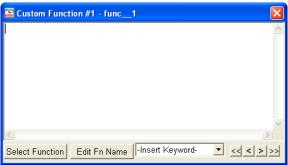
TBASIC code is entered into the custom function, which allows the possibility of total control of all of the PLCs functions and hardware.
