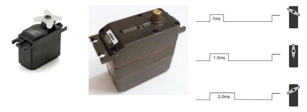
Figure 11.3 RC Servo and Control Signal
