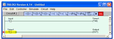
Figure 4.2: Completed Timer Circuit
