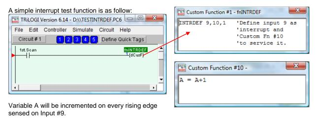
**Note:** Since inputs 3 to 6 can also be used as other special inputs such as High Speed Counter (HSC) inputs and/or Pulse Measurement (PM) as described in Chapter 6, 7 and 8, if these inputs are defined as interrupts using the INTRDEF statement, then they will lose their other special function. I.e., they can only be defined either as a HSC/PM or as an interrupt input and not both.
