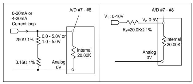
Converting 20mA current-loop to 0-5V
