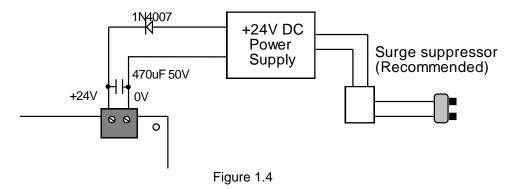
If the AC main is affected by nearby machines drawing large amounts of current (such as large three-phase motors), you should use a surge-suppressor to prevent any unwanted noise voltage from being coupled onto the FMD1616-10 power supply. The required current rating for the power supply depends mainly on the total output current, taking into consideration the peak current demand and the duty cycle of the operation.
