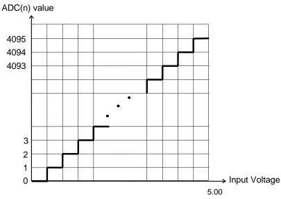
Figure 5.1 Transfer Function for 12-bit ADC.
