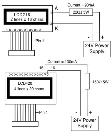
Figure 1.8 – Wiring of LCD216 and LCD420 backlight.
