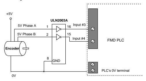
Figure 7.2 Interfacing 5V type Rotary Encoder
