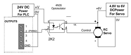
Figure 11.5 Opto-Isolated Interace to RC Servo
