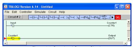
Figure 4.4: Completed Counter Circuit
